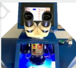
Step 10 adjust the welding point with the cross center of the microscope 1--Up and Down 2--move with the 45° line 3--Left and Right
